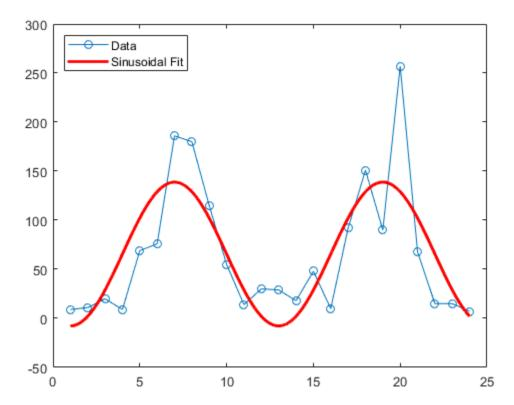
Use the lscov function to compute statistics on the fit, such as estimated standard errors of the coefficients and the mean squared error:
