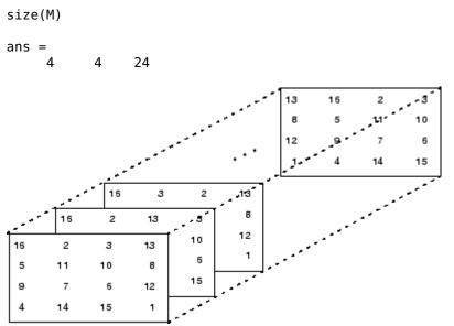
stores the sequence of 24 magic squares in a three-dimensional array,  ${\tt M}.$  The size of  ${\tt M}$  is
