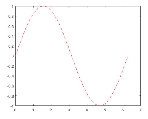
'r - - ' is a *line specification*. Each specification can include characters for the line color, style, and marker. A marker is a symbol that appears at each plotted data point, such as a +, o, or \*. For example, 'g:\*' requests a dotted green line with \* markers.
