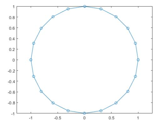
The axis equal command makes the individual tick-mark increments on the *x*- and *y*- axes the same length, which makes this plot more circular in appearance.
